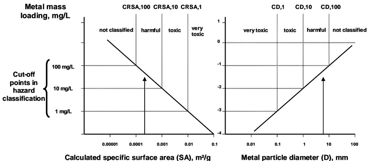
**Figure 8:** Illustration of hazard identification line and resulting self-classification levels for a metal with (a) various calculated critical reference surface area values and (b) corresponding diameters (CD) (adapted from Skeaff et al, 2000)
