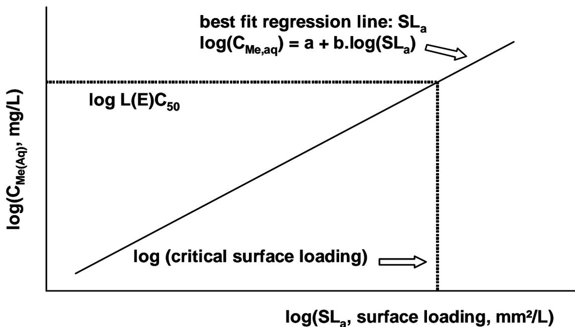
**Figure 7:** Determination of critical surface loading from regression line of log concentration of dissolved metal versus log surface loading (adapted from Skeaff et al, 2000)
