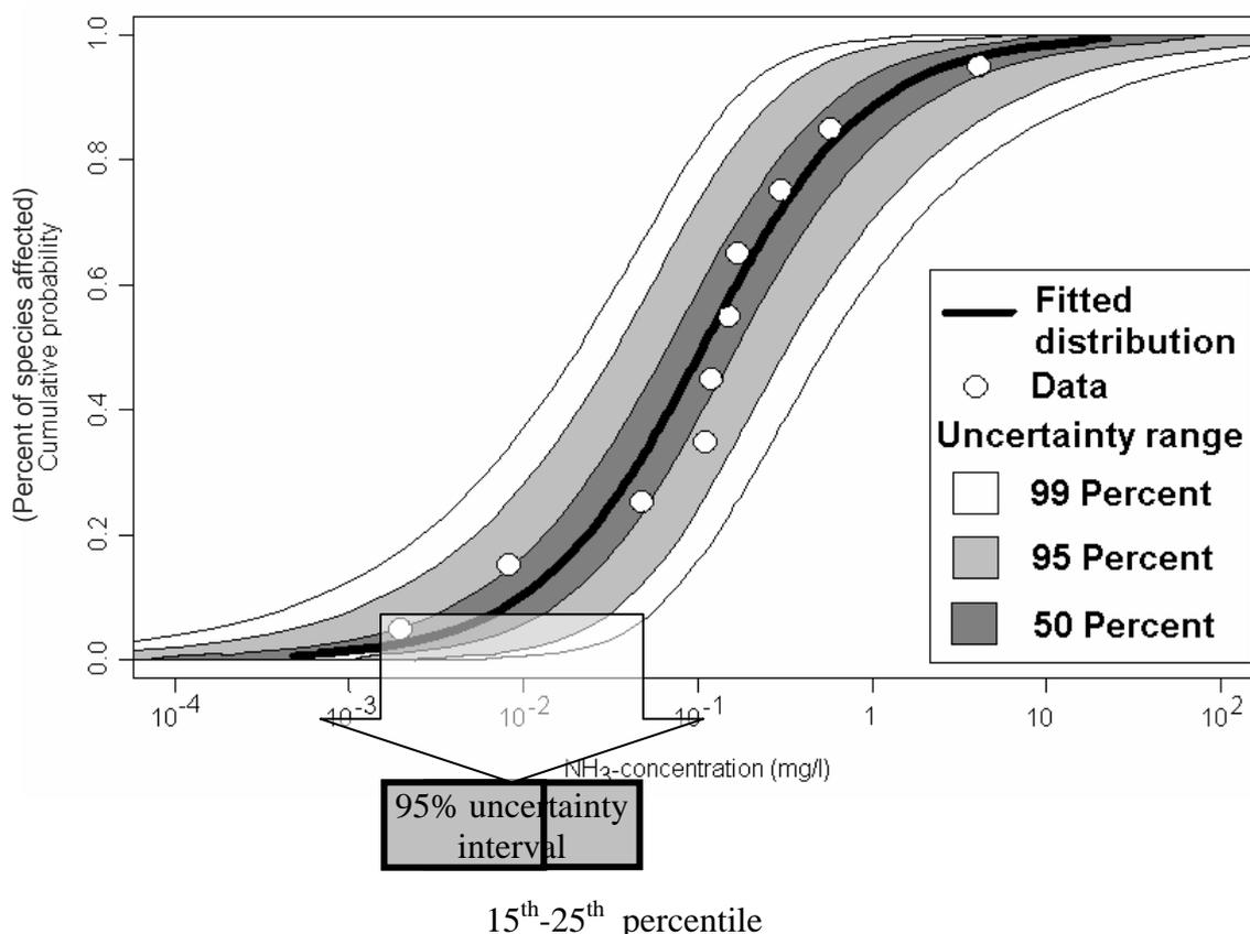
**Figure 2:** Example of a SSD (Species Sensitivity Distribution - log logistic distribution) with uncertainty band and an HC<sub>15</sub>- HC<sub>25</sub> (Hazardous Concentration at 15-25 %) as possible ecotoxicity threshold for classification purposes.
